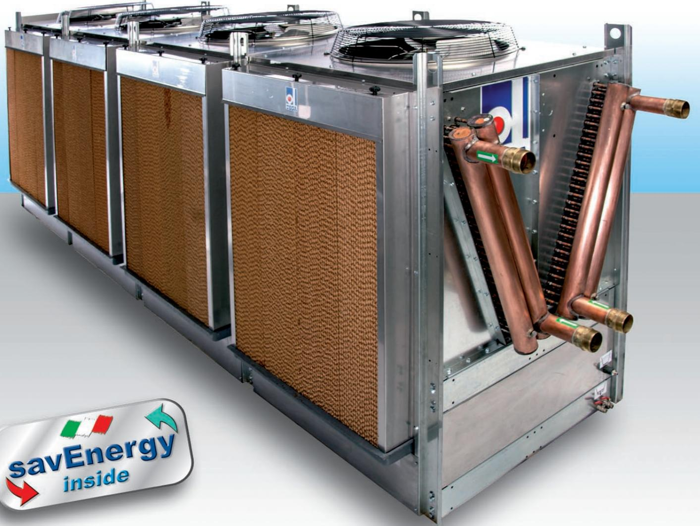
In climates where the temperature is unfavorable for the installation of an **ECOENERGY SYSTEM**, alternative options are: (1) Cooling Towers, which have serious problems due to the large consumption of water with consequent tartar and sludge deposits that require frequent cleaning or (2) **Dry Cooler** plants with auxiliary cooling systems with direct water nebulization in the radiator or adiabatic systems with evaporation panels, consequently with water waste.
